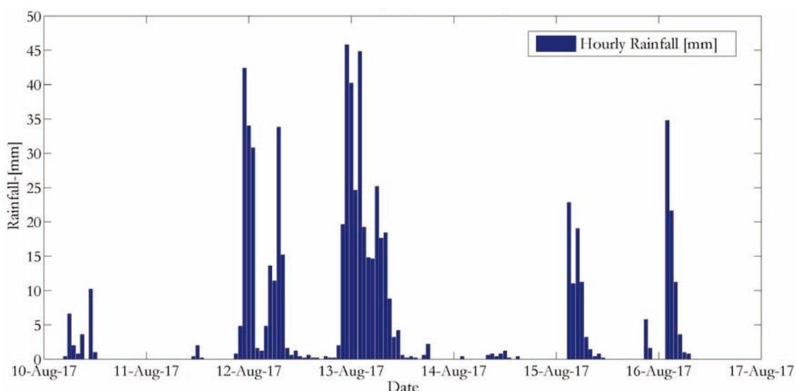
**Figure 4.4(a)** Rainfall recorded at Chepang station during 2017 flood
