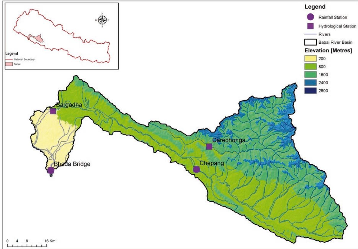
**Figure 1.7** Babai River basins in West Nepal with flood forecasting station at Chepang and Bhada bridge
