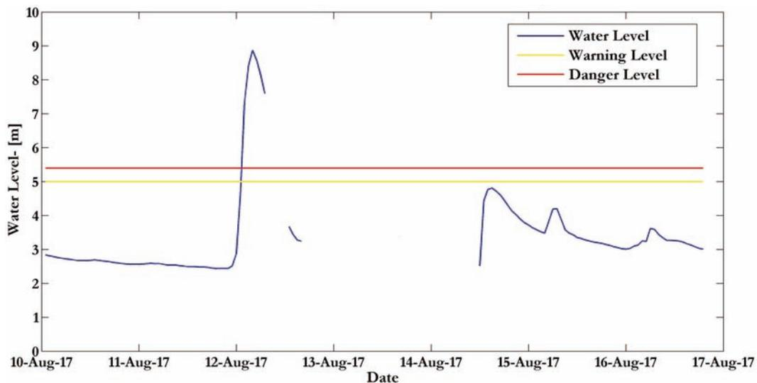
**Figure 4.3(a)** Water level of West Rapti River at Kusum station during 2017 flood
