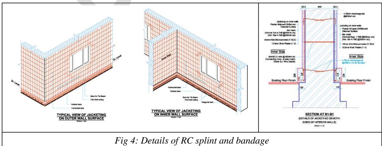
Fig 4: Details of RC splint and bandage
