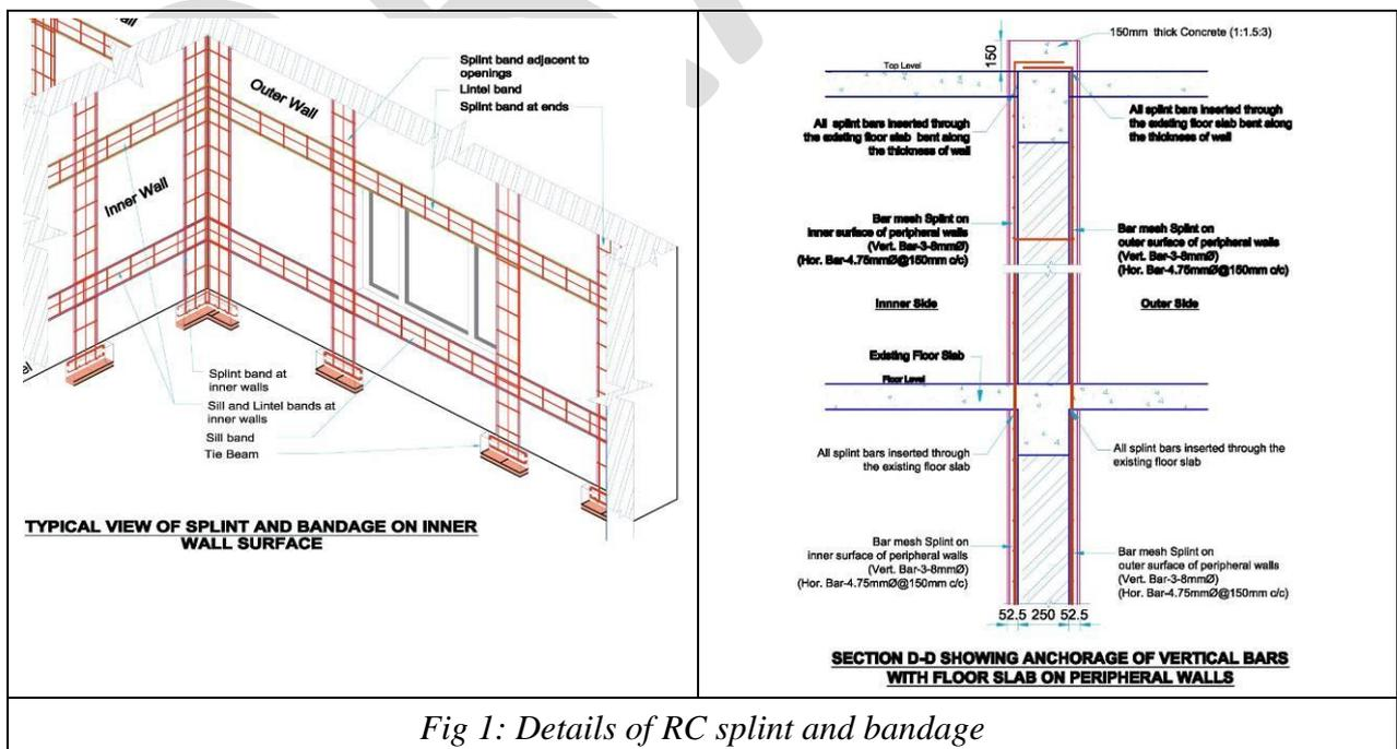
Fig 1: Details of RC splint and bandage
