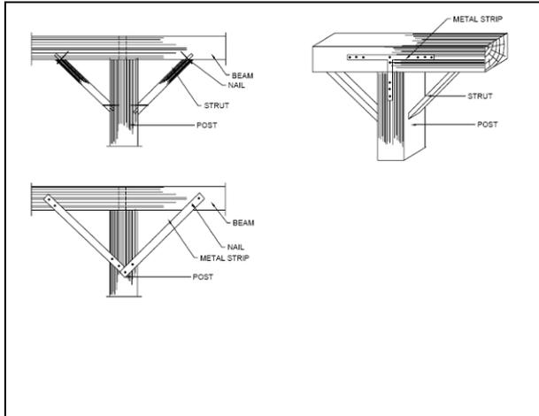
*Fig 16: Improvement of roof connections*
