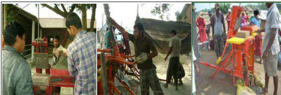
Figure 13 Pouring mixed soil, handling machine and CSEB production at Morang district
