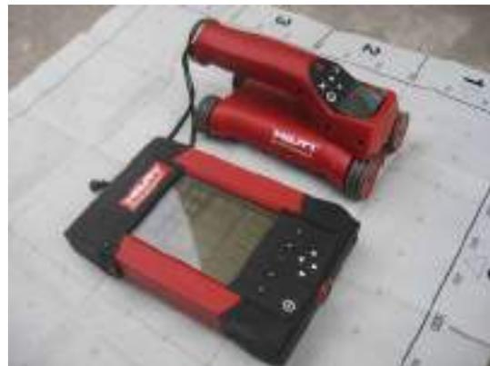
**Fig 2. (b) Ferro-scan Detector**
