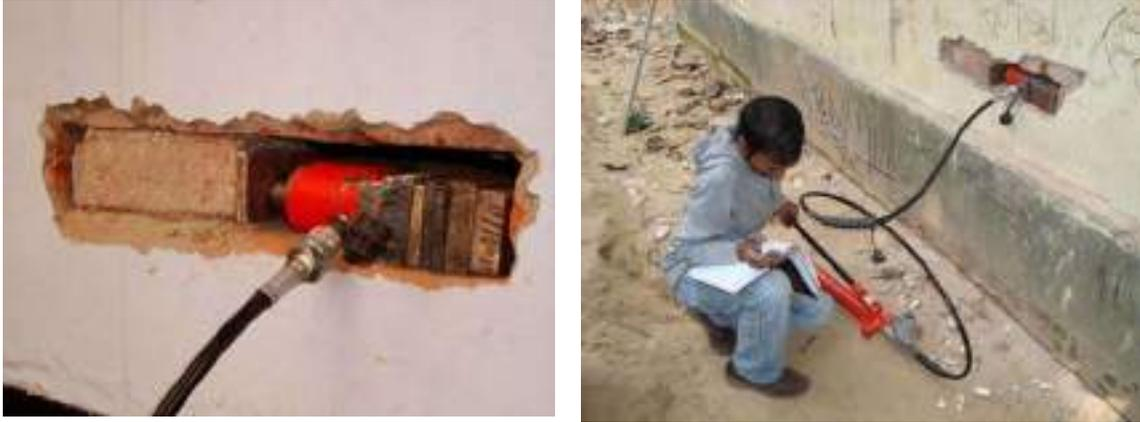
**Fig 3. Test Set up for In-Situ Shear Test**
