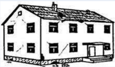
Grade 2: Moderate damage
