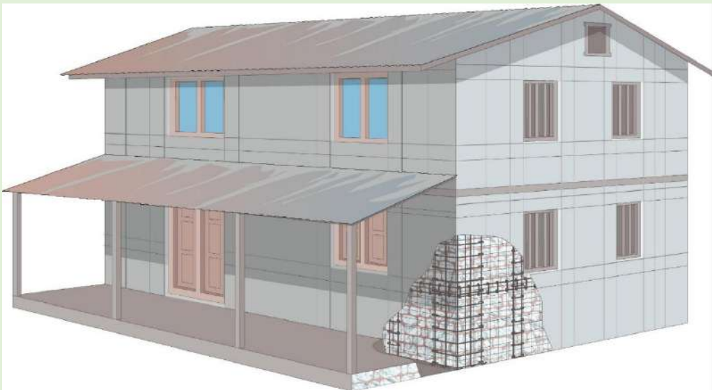
Retrofitting using rebar with concrete Splint-bandage and GI wire mesh Jacketing (Stone Masonry)
