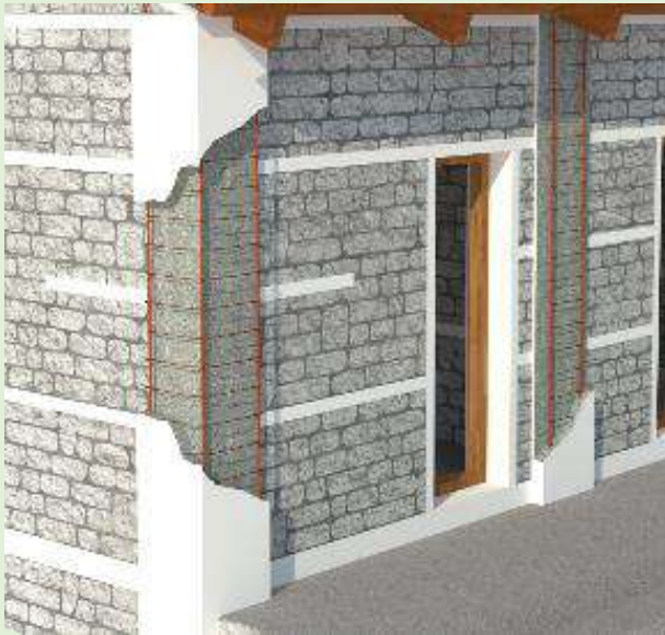
G I wire mesh anchored R C splint
