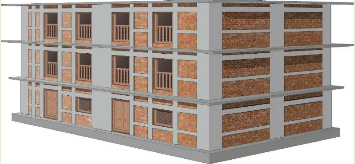
Retrofitting using rebar with concrete Splint-bandage and GI wire mesh Jacketing (Brick Masonry)
