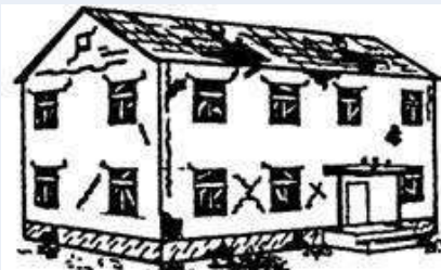
Grade 3: Substantial to heavy damage
