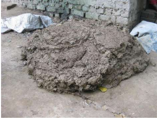
(Mud plaster prepared by mixing mud and pieces of thatch and straw)
